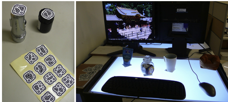
Figure 6.1 The iCon system: Tangible objects are tracked around the desk.
