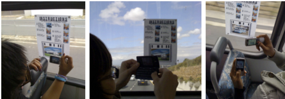
Figure 19.7 The mobile Snap 'n Grab system in use on public transport. Taking a photo of any desired item and sending the photo via Bluetooth to a mobile media library phone causes the requested media to be sent back in response.
