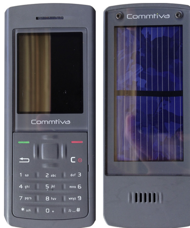
Figure 19.4 Commtiva’s Sola handset charged by solar panels on the reverse. While an admirable attempt at designing a handset specifically for developing regions, the handset was ultimately a commercial failure.
