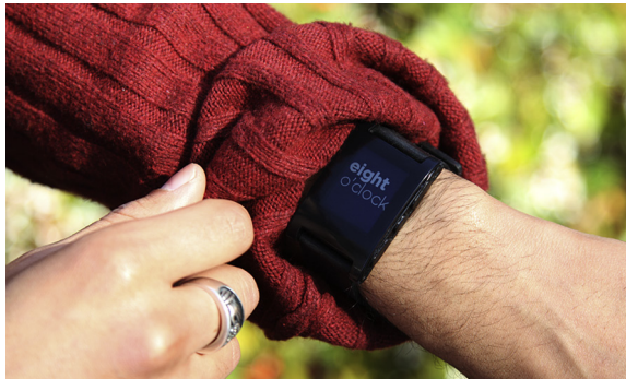
Figure 9.2 The Pebble e-paper watch. The watch pairs with a phone using Bluetooth, then displays alerts at a glance.
