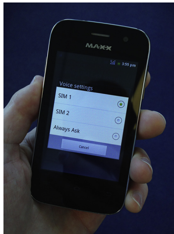
Figure 19.2 Indian manufacturer Maxx Mobile makes several Android phones that support hot-swapping of SIMs. Multi-SIM handsets are becoming increasingly popular in developing regions, as they allow phone users to mix and match networks to reduce costs.
